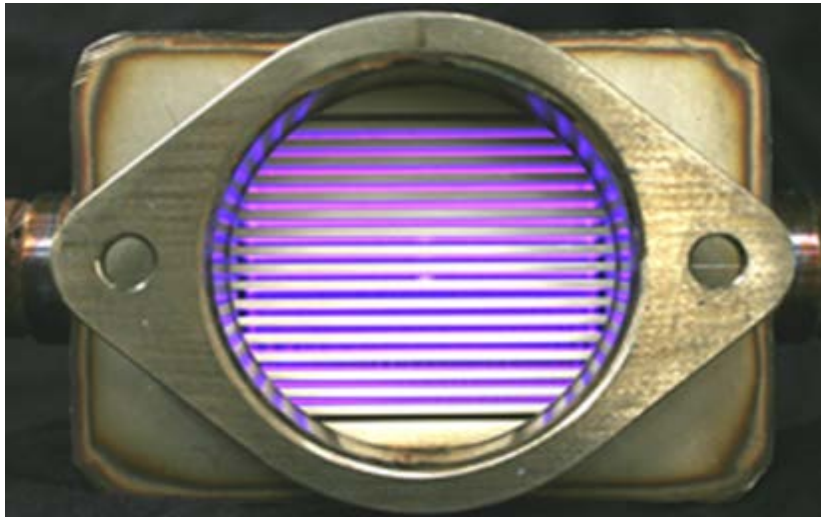
Home made Ozone (GREMI) reactor Using Air into the intake port
